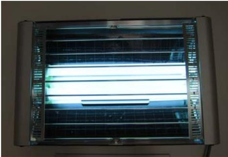
**Figure 5:** Ultraviolet light trap.
